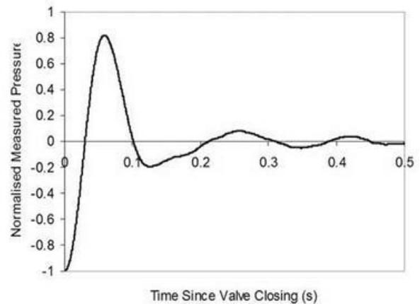
The adjacent graph shows a typical pressure wave caused by closing a valve in a pipeline. This pressure wave can cause major problems, from noise and vibration to **pipe collapse**.
