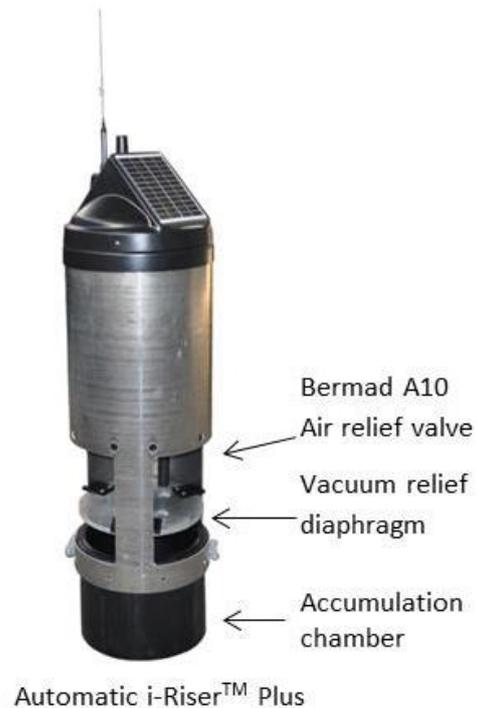
The i-Riser™ Plus incorporates a large orifice area of 5028mm<sup>2</sup> to provide an air intake, vacuum release capacity greater than that of a typical 3” Combination full port Air Relief Valve (ARV).
