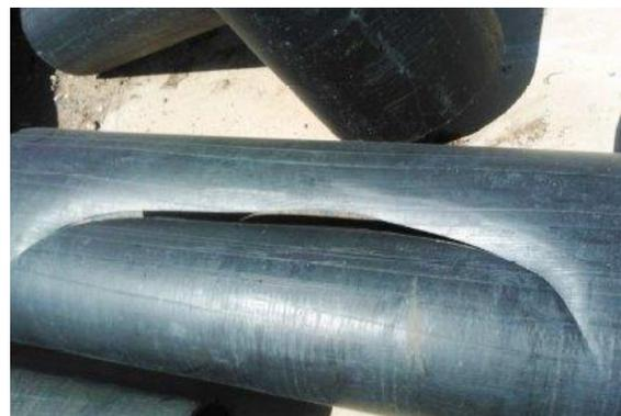
Evidence from installed systems indicates that a number of pressurised Pipe and Riser **pipeline failures**, (pipe collapsing and splitting) are a direct result of dynamic pressure changes creating a negative pressure (vacuum) condition.
